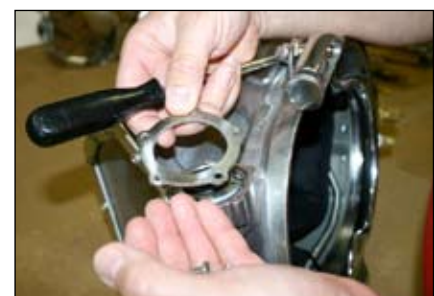
Step 6: Remove regulator cover.
