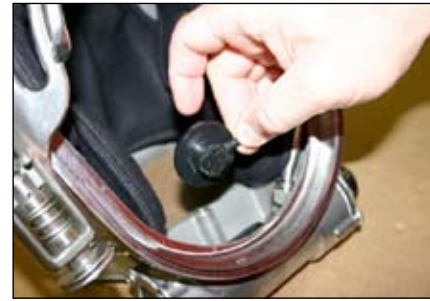
Step 14: Place Velcro tab on base of microphone.
