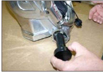
Step 11: Install free flow plug in helmet shell. Ensure Velcro strip is facing inward.
