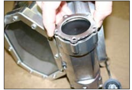
Step 12: Replace regulator cover.
