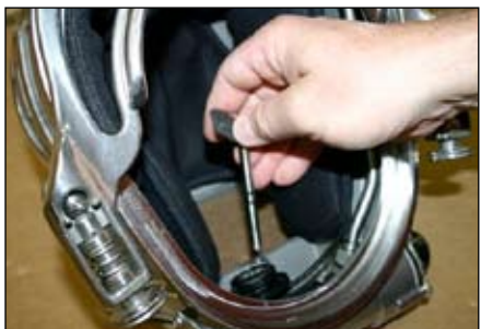
Step 16: Reinstall NCD.
