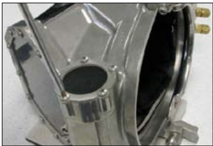
Step 13: Tighten exhaust valve cover screws using a Phillips #3 screwdriver to 45 in.lbs (5 Nm).
