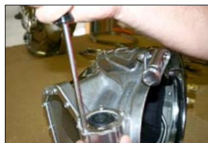
Step 5: Remove exhaust valve cover screws using a Phillips #3 screwdriver.
