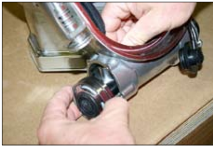
Step 7: Remove regulator.
