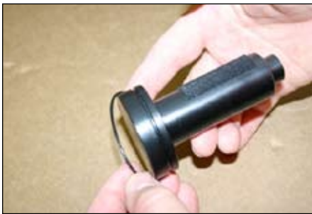
Step 10: Lubricate and install o-ring on outside of free flow plug. Place Velcro strip on barrel.
