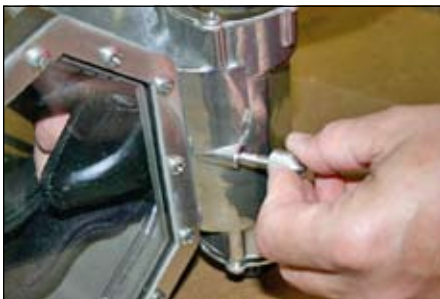
Step 1: Remove nose clearing device (NCD) knob.
