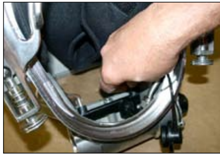
Step 8: Remove defogger train.
