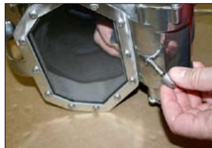
Step 17: Place NCD knob on NCD to secure in place.
