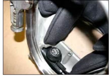
Step 15: Place microphone on free flow plug.
