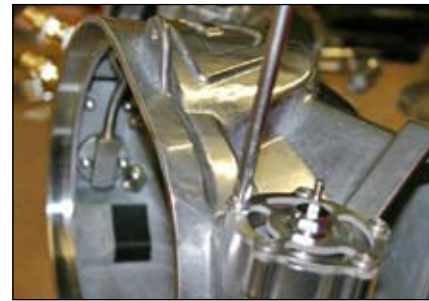
Step 3: Unscrew exhaust valve cover screws using a Phillips #3 screwdriver.
