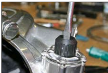
Step 16: Tighten knob nut until snug using a 3/8" flat blade screwdriver.
