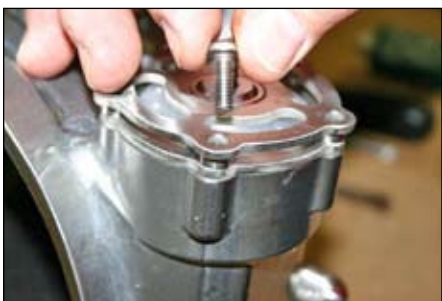
Step 13: Insert exhaust valve cover screws and tighten by hand.
