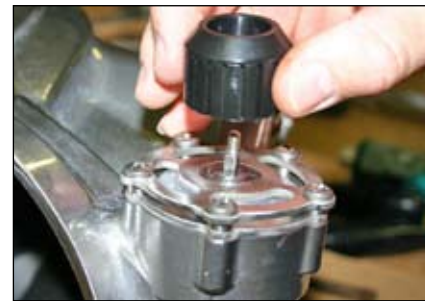
Step 15: Replace free flow knob, knob spring and knob nut.
