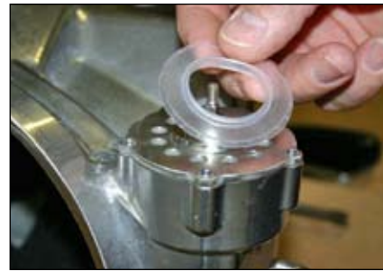
Step 9: Place flapper exhaust valve onto the dual exhaust seat. DO NOT LUBRICATE.
