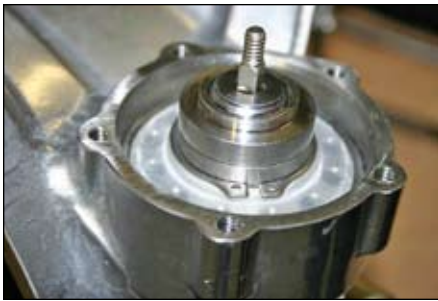
Step 7: Dual exhaust bushing installed onto free flow valve stem.
