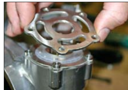
Step 12: Place exhaust valve cover on top of spacer rings.
