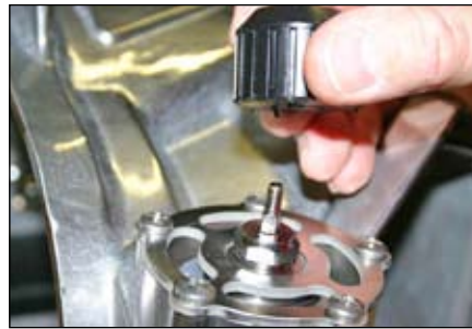
Step 2: Remove free flow knob, knob spring and knob nut.
