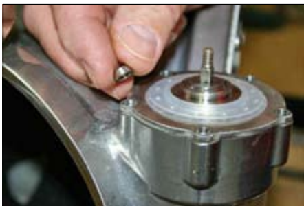
Step 10: Place all spacer rings onto the dual exhaust seat.
