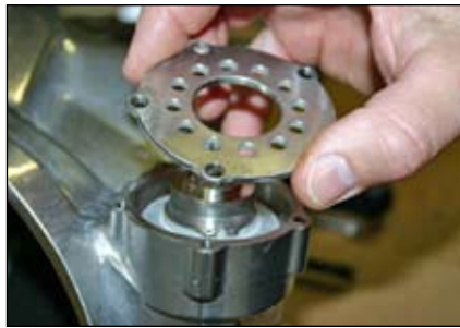
Step 8: Place dual exhaust seat over the dual exhaust bushing.
