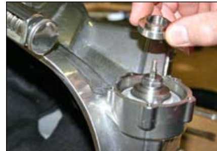
Step 6: Place dual exhaust bushing over free flow valve stem.
