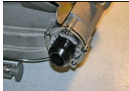
Step 17: Double exhaust installed.
