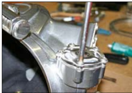
Step 14: Tighten screws using a Phillips #3 screwdriver to 45 in.lbs (5 Nm).
