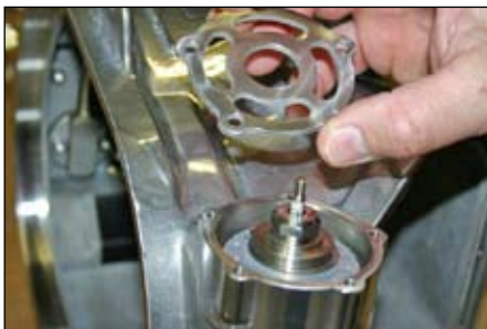
Step 4: Remove valve exhaust cover.
