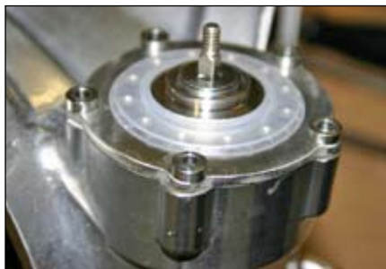
Step 11: Spacer rings in place.
