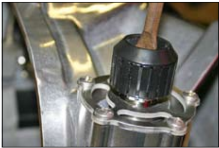
Step 1: Unscrew knob nut with a 3/8" flat blade screwdriver.
