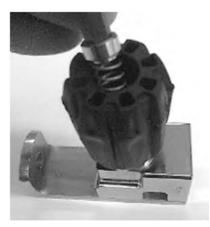
9. Put the O ring (12) over the 1/2" thread on the connector (11).
