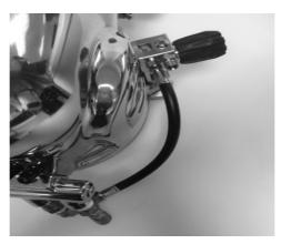
9. Connect the MP supply hose from the 1st stage regulator on the EGS/bailout cylinder to the 9/16" inlet connector of the side block valve. Use a torque wrench and 11/16" crowfoot fitting to apply 5 Nm (44 in.lbs) of torque to the hose female end.
