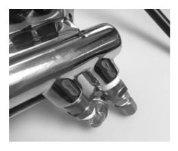
8. Connect the MP short hose AP0203/1-0.27M to adaptor AP2541 while holding adaptor still with 7/8" spanner use torque wrench and 11/16" crowfoot fitting to apply 5Nm (44 in.lbs) to AP0203/1-0.27M
