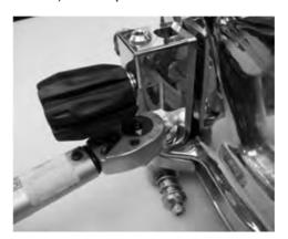
6. Connect the MP short hose AP0203/1-0.27M male end to the 3/8" outlet of the helmet side block valve. Use a torque wrench and 9/16" crowfoot fitting to apply 5 Nm (44 in.lbs) of torque to the hose male end.
