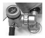
Vent air from the unitby purging the valve or from an attached regulator.
