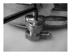
2. Re-use the grower washer 400120 on the new hexagonal head screw 530006 included in the kit.
