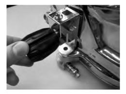
4. Place the hexagonal head screw with grower washer through the side block valve, helmet mounting hole and into the threaded latch hole.
