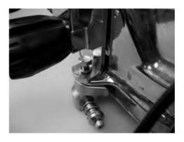
5. Use a torque wrench and 1/2" crowfoot fitting to tighten the hexagonal head screw 530006 (13) and apply 15 Nm (133 in.lbs) of torque.
