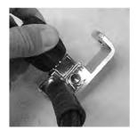
NOTE: If there's no gas flow, check gas supply. If supply has no faults check helmet side block valve for blockages / debris.
