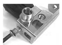
Assembly for the helmet side block valve is now complete
