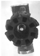
Press the spring (7) onto the retaining nut (8). Secure the hand wheel (6) with the retaining nut (8). Use a torque wrench with 8mm hex key to apply 5 Nm (44 in.lbs) of torque to the retaining nut (8).
