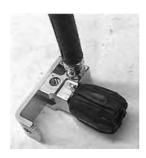
2. Ensure hand wheel is in the closed position on the helmet side block valve. Slowly turn on air supply then slowly open helmet side block valve, an audiblegas flow should be present. Close helmet side block valve hand wheel
