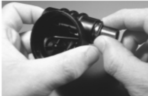
Figure 41 - Installation of valve body O-ring
