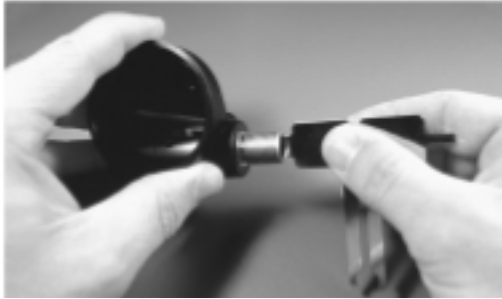
Figure 49 - Crown pre-set adjustment
