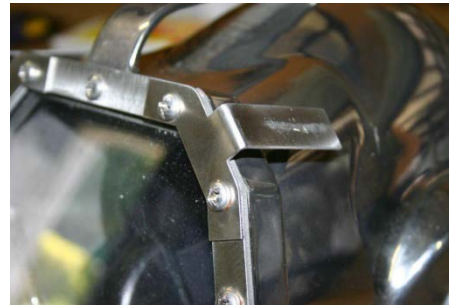
Step 6: Left hand Bracket installed
