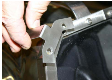
Step 2: Line up Bracket holes with Helmet Retainer holes
