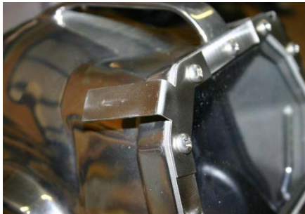
Step 4: Right hand Bracket installed
