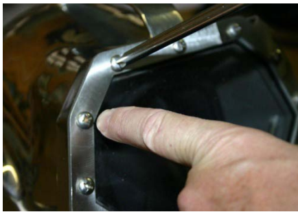
Step 1: Remove 2 screws from top corner of Helmet
