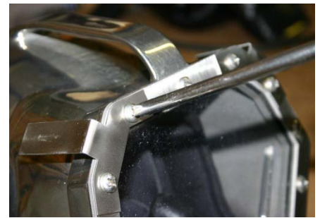
Step 3: Replace the 2 screws and tighten until snug
