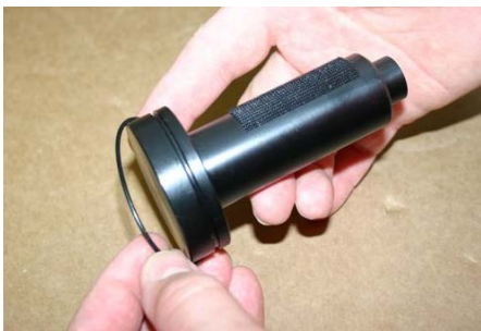
Step 10: Lubricate and install O-ring on outside of Free Flow Plug. Place Velcro strip on barrel.
