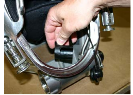
Step 9: Remove Free Flow Barrel
