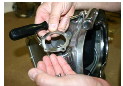
Step 6: Remove Regulator Cover
