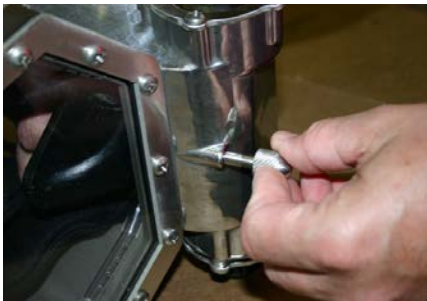
Step 1: Remove Nose Clearing Device (NCD) Knob
