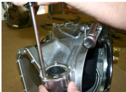
Step 5: Unscrew Regulator Cover
