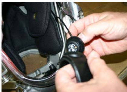
Step 4: Remove Microphone
