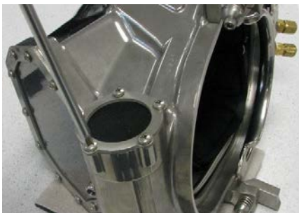
Step 13: Tighten Regulator Cover screws until snug
