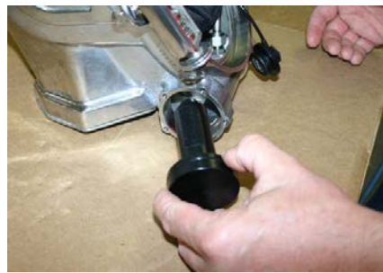
Step 11: Install Free Flow Plug (with O-ring) in helmet
