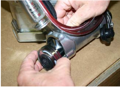
Step 7: Remove Regulator
