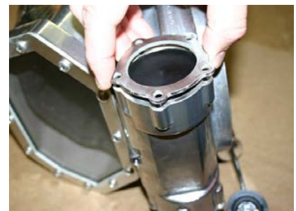
Step 12: Replace Regulator Cover
