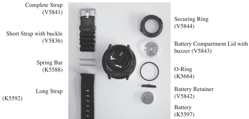
Fig. 5.1 Instrument parts. The code after the name stands for spare part order number.
