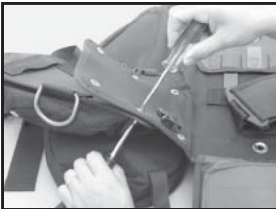
Figure 15 - Remove both bolts using a Phillips screwdriver and 3/8" nutdriver or wrench
