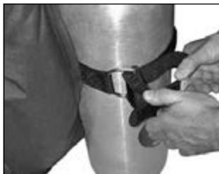
4. Pull the cam buckle closed so that it lies flat against the cylinder. Secure the end of the cylinder band with the hook & loop attachment.
