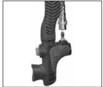
2. Remove the port plug from a MP port on the regulator using an appropriately sized wrench.
