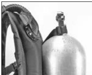
2. While holding the cylinder secure, pull the free end of the cylinder band until there is a very tight fit between the pack and the cylinder.
