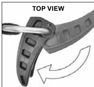
3. Insert band through the metal D-ring, then through the middle slot.
