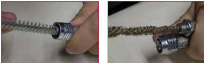
5 Clean the ends of the hose with hot soapy water in order to remove dirt residues and grease. Rinse the ends of the hose under running water. Rinse the inside of the hose by circulating tap water through it.
