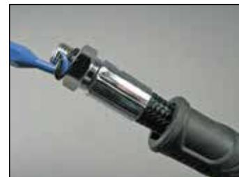
**2** To perform complete cleaning, you will need to use brushes and swabs: soft bristles (nylon bristle brush) and stiff bristles (brass) for when corrosion is evident. Also, a soapy hot water bath is necessary to remove any traces of grease.
