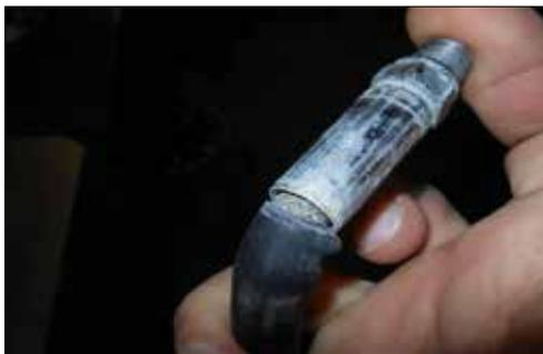
**2** Examine the length of the hose looking for blisters, hernias, heavy abrasion or cuts, excessive scratching, broken or frayed nylon braiding.
