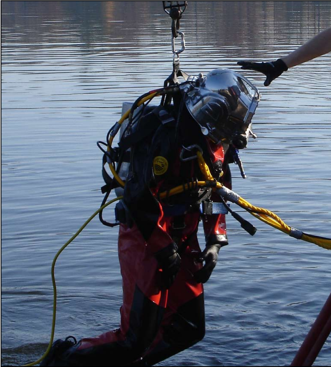
Photograph shows a surface-supplied diver being recovered from the water in an emergency using the Personal Diver Harness (PDH) attached to the recovery hoist.
